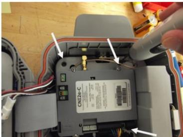
Loosen screws in 3 positions
