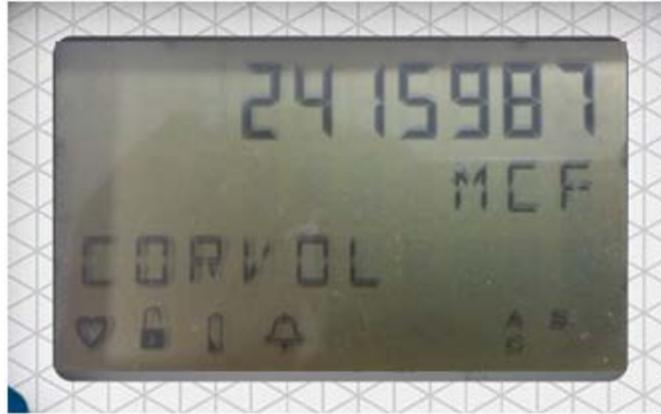
1. Top line of LCD display indicates the totalized corrected volume value.
