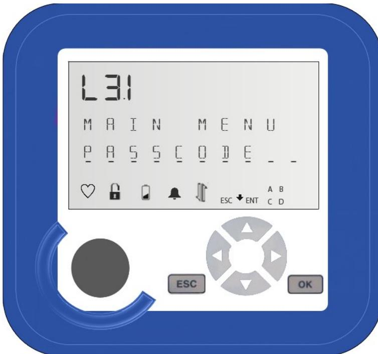
3. To access the passkey screen, in level 3 mode press **OK**. The following appears on the display.
