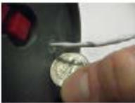
The one inch additional length ensures that the probe bottoms out at the end of the thermowell.
