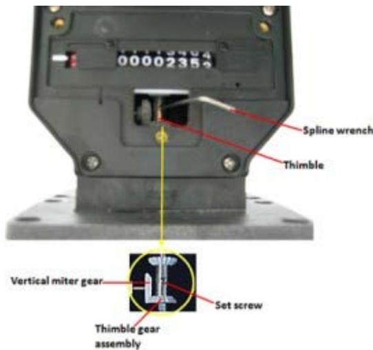
2. Loosen the **Set screw** on the Thimble gear assembly.
