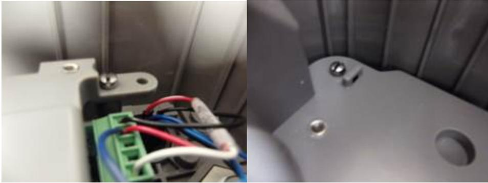
3. Re-install Human Factor cover tightening the screws to 9 +/- 1 in-lbs of torque at these locations. Ensure power cable is routed in the orientation shown for battery connection.
