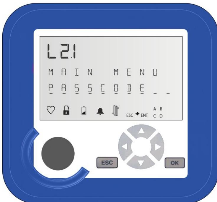
3. To access the passkey screen, in level 2 mode press **OK**. The following appears on the display.
