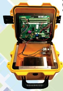
Eagle offers a Portable version of the EPR for pressure testing in the field. Offering pressure measurement in locations of the gas system where permanent installations are not practical or required.
