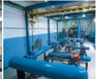
High Pressure Flow Loop; up to 62 bar (900 psi)
