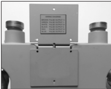
Figure 20: Properly positioned mounting bracket
