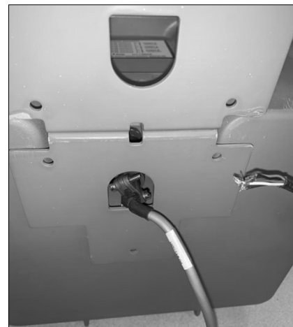
Figure 24: Properly positioned mounting bracket
