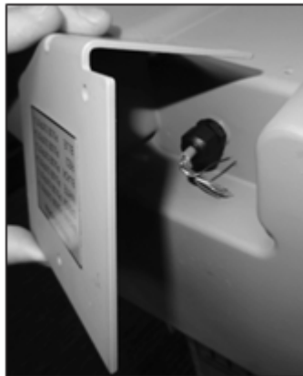
Figure 34: Pulse output cable under the protective plate
