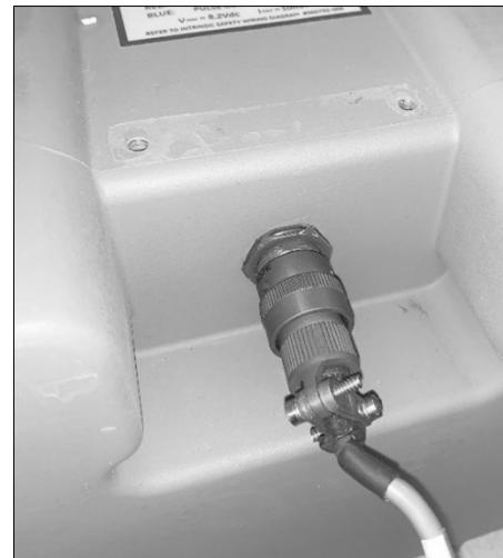
Figure 23: Pulse output cable plugged into connection
