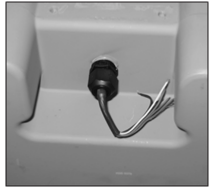
Figure 18: Pulse output cable on backside of meter
