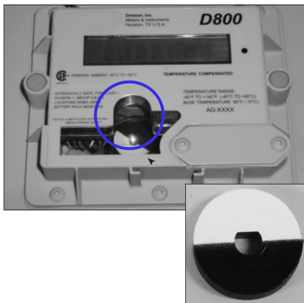
Figure 3: RPM Wheel location under cover in meter
