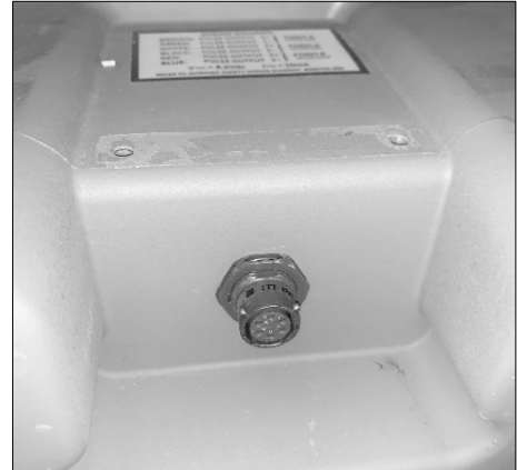
Figure 22: Pulse output cable connection on backside of meter
