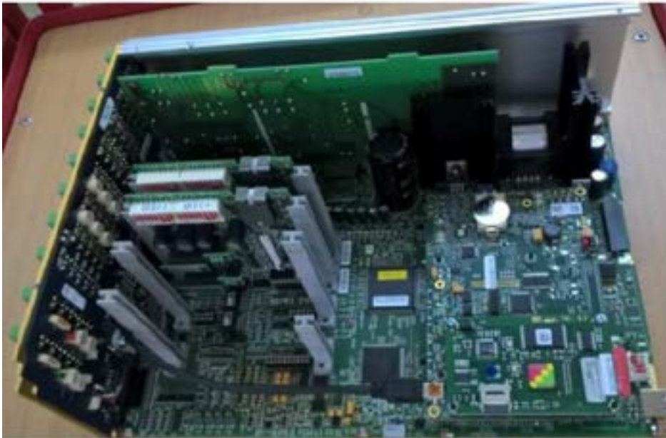
Fig. 8.21: Slot for the option card with COM 6 and 7 of the ERZ 2000-NG
