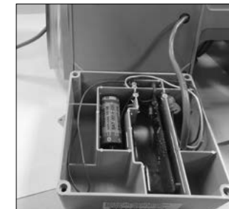
Figure 25- Tuck extra cable into a pocket
