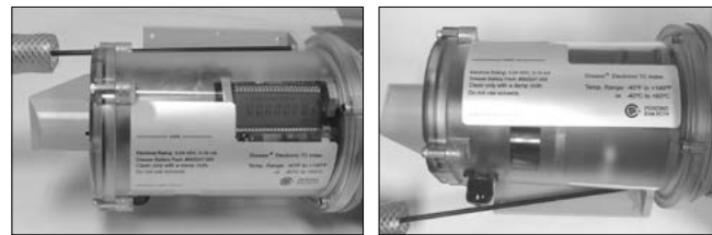
Figure 8 - Remove screws to AMR bracket
