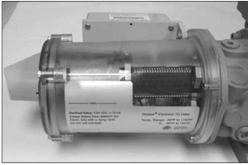
Figure 29 - Top inlet: notice the space between the ETC label and the bracket
