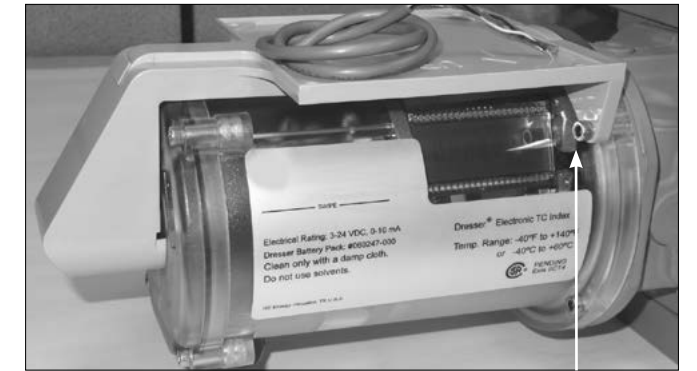
Figure 15 - Insert the 7/8" (long) screws 7/8" screws (one not shown)
