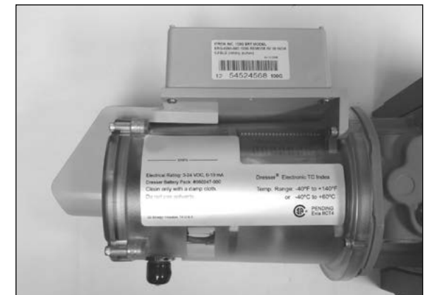
Figure 28 - Side inlet: notice the close positioning of the ETC label to the bracket
