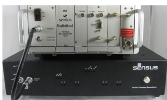
A Vehicle Transceiver Unit (VXU) is required for dual reading capability.
