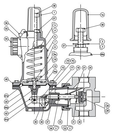
Adjust set-point (outlet pressure) by turning adjustment screw (58). Turn clockwise to increase and counterclockwise to decrease. After making the necessary adjustments, tighten nut (57). Do not adjust when regulator is closed (no flow). Only adjust when gas is flowing through regulator (approximately 250 SCFH).
