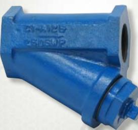
Sure Flow threaded strainers in Cast Iron feature a machined seat which ensures a perfect fit for the removable, stainless steel screen. All sizes come complete with NPT blow-off with plug, which can be replaced with a ball valve for on-line blow-down of particulate.
