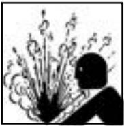
**CAUTION: THE METER END COVER IS PRESSURIZED. Bleed off the line pressure before removing the oil fill or drain plugs from the meter.**
