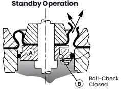
Both illustrations show the monitor in the downstream position. When installed this way, the 441-X57 is usually set for an outlet pressure 4 to 6 psi higher than the operating regulator and thus is wide open during normal operation.
