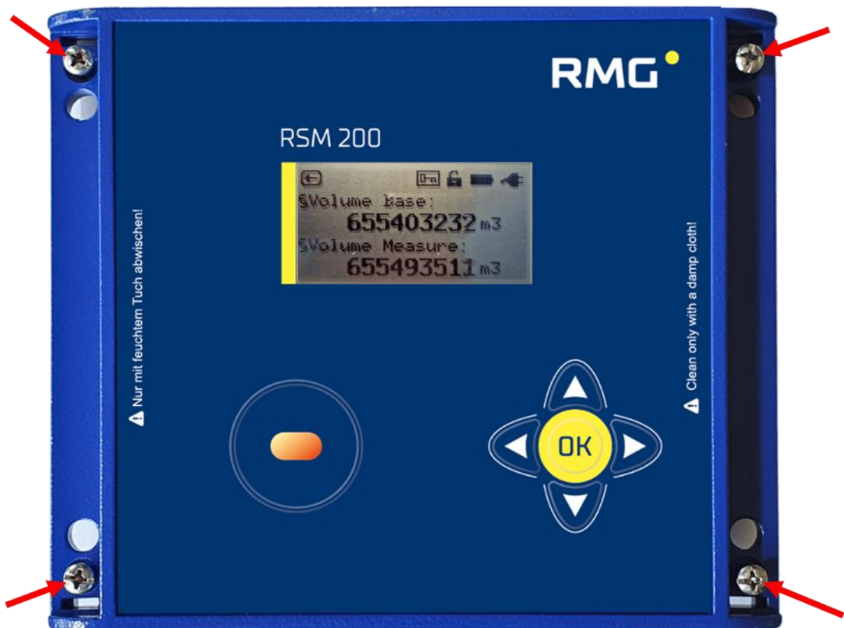
Figure 9: Unscrewing the screws to open the cover
