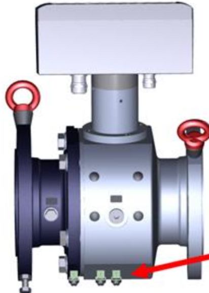
Figure 13: Grounding of the measuring instrument
