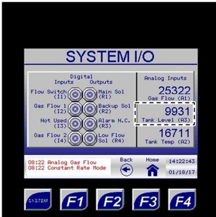
This analog signal is the raw count coming into the odorizer after the signal has been converted from milliamps. This value will vary according to the output from the level transmitter.
