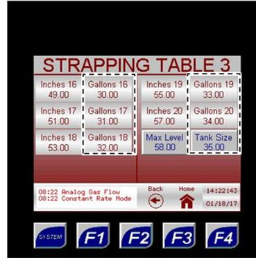
The right column of each table displays the tank volume in US gallons per inch.
