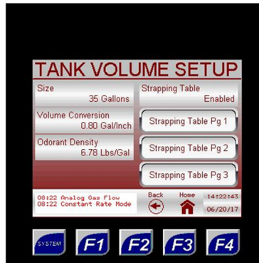
Figure 40: Odorant Tank – Tank Volume Setup
