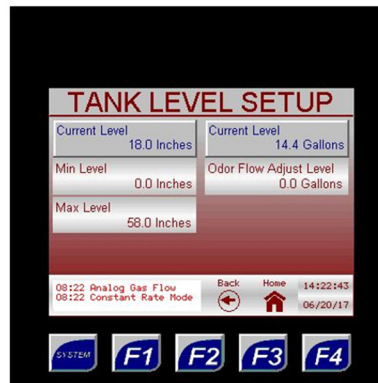
Figure 39: Odorant Tank – Tank Level Setup
