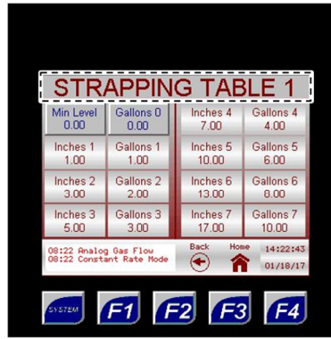
Figure 41: Tank Volume Setup – Strapping Tables
